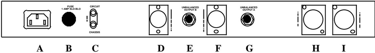
**A IEC MAINS SOCKET** Standard IEC mains socket (120/240 VAC)
