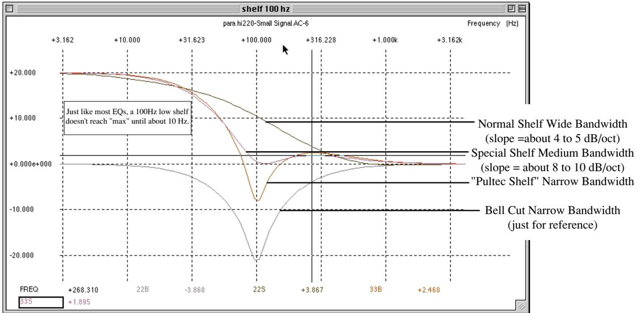
22Hz and 33Hz are different shelves when the Bandwidth is Narrow
