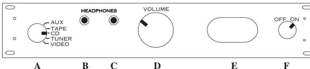
**A - INPUT SELECT** - 5 Position switch for input selection. Each input is electrically identical. The RECORD OUT directly follows this switch. There is no buffer amp to isolate the effects of loading and cable capacitance so we recommend disconnecting any interconnect cables from the RECORD OUT if you are not recording.
