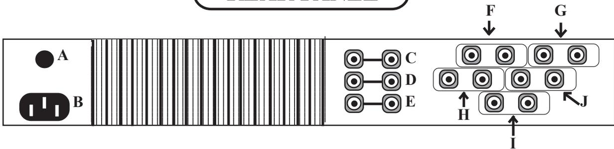
**A) MAINS FUSE** - Depending on your local power outlet's voltage, replace with 3A SLO-BLO fuse (120 V) or 1.5A SLO-BLO fuse (230V).
