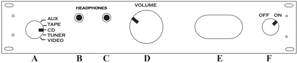
**A) INPUT SELECT** - 5 Position switch for input selection. Each input is electrically identical. The RECORD OUT directly follows this switch. There is no buffer amp to isolate the effects of loading and cable capacitance so we recommend disconnecting any interconnect cables from the RECORD OUT if you are not recording.
